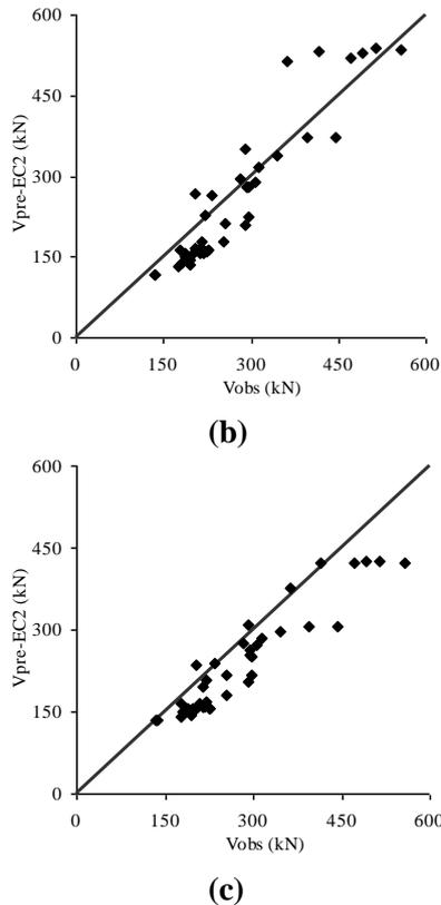
**Figure 1: Comparison of observed shear strength to the predicted shear strength by (a) ACI, (b) EC2 and (c) CSA.**
