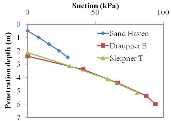
Figure 2: Required suction for penetration of caissons in sandy soils
