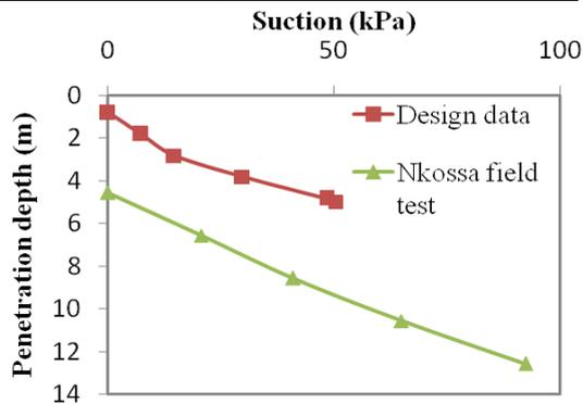
**Figure 3: Required suction during penetration in clayey soils**
