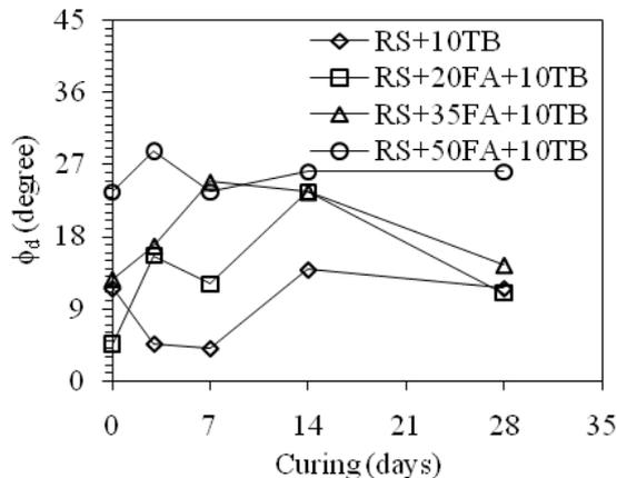
Figure 10: Variation of  $\phi_d$  with curing RS+fly ash+10TB mixes
