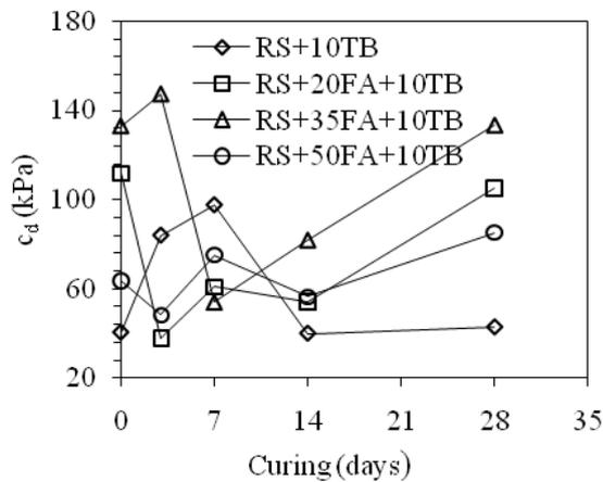
Figure 9: Variation of  $c_d$  with curing for RS+fly ash+10TB mixes
