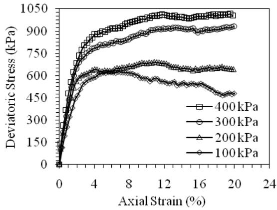
Figure 2: Deviatoric stress-axial strain plots for RS+35FA mix at 7 days curing
