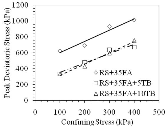
Figure 5: Peak deviatoric stress-confining stress plots for RS+35FA+tyre buffings mixes at 7 days curing
