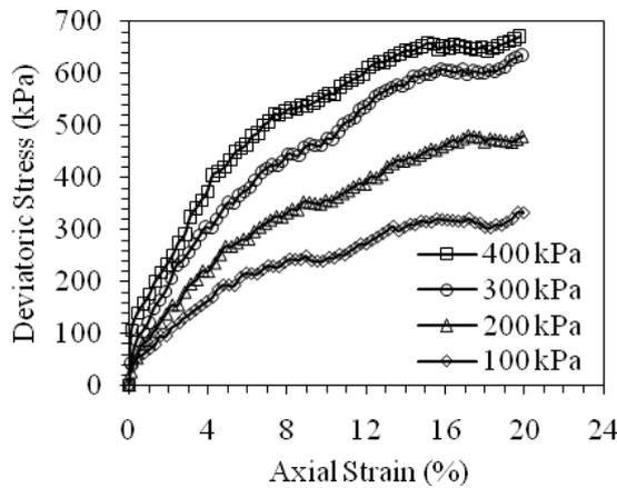
Figure 3: Deviatoric stress-axial strain plots for RS+35FA+5TB mix at 7 days curing
