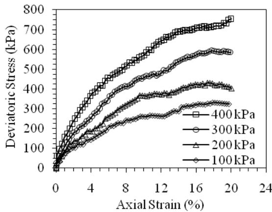
Figure 4: Deviatoric stress-axial strain plots for RS+35FA+10TB mix at 7 days curing
