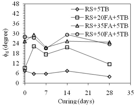
Figure 8: Variation of  $\phi_d$  with curing for RS+fly ash+5TB mixes
