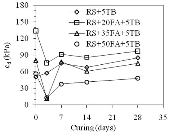
Figure 7: Variation of  $c_d$  with curing for RS+fly ash+5TB mixes
