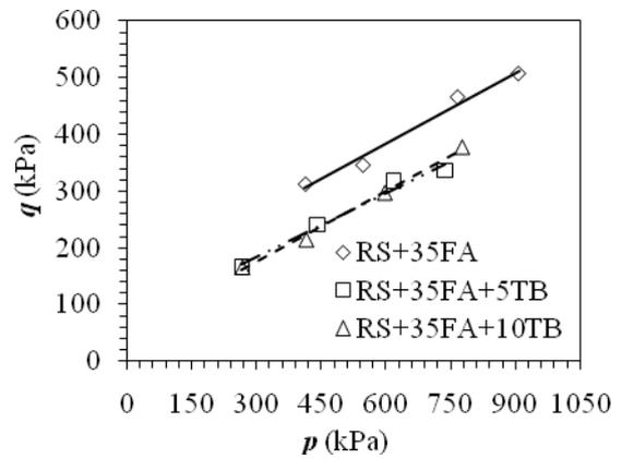
Figure 6:  $p$ - $q$  plots for RS+35FA+tyre buffings mixes at 7 days curing
