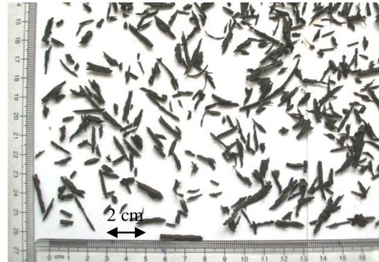
**Figure 1: Rubber fibers used (retained between 4.75 and 2 mm size sieves)**
