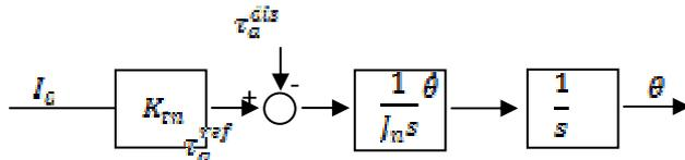
Fig. 1: Control diagram of the motor with the disturbance torque
