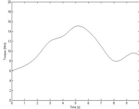
Fig. 10a: Load torque profile of the left wheel
