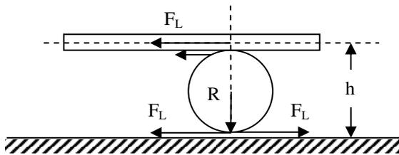
Fig. 5: Components of the  $F_L$  in the perpendicular plane
