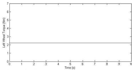
Fig. 12a: Load torque of the left hand side wheel
