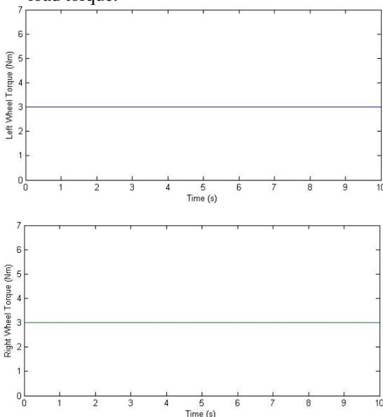
Fig. 9: Load torques of the two wheels when in normal operation.
