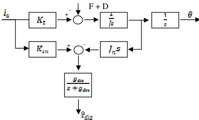
Fig. 2: Control Diagram of Disturbance Observer
