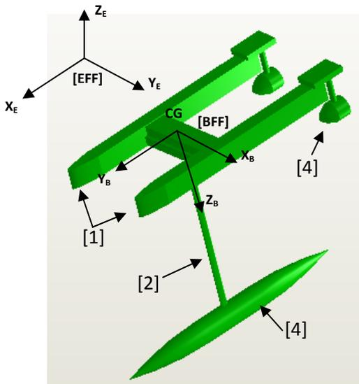
**Fig.1:** design of the ASV (where [1] hulls, [2] vertical strut, [4] Gertler body, and [4] propellers) and Coordinate frames
