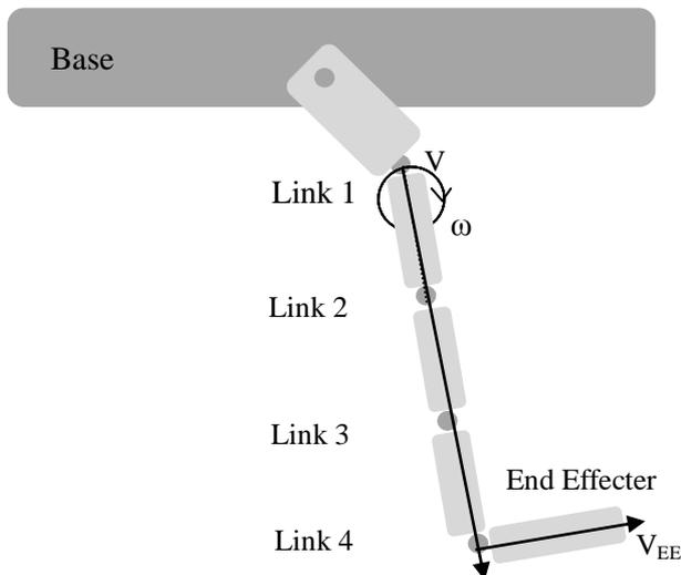
Fig.02- An example of a Kinematic Chain of a robot limb
