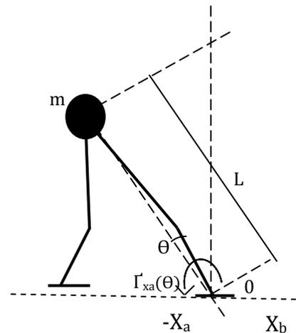
Fig.05- Robots Inverted Pendulum model applied to two limbs
