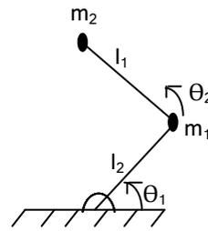
Fig.04- Manipulator Control- Joint space equation of motion
