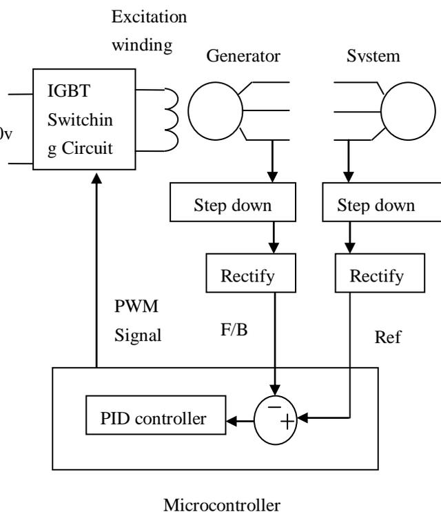
Fig 2: Voltage controlling block diagram
