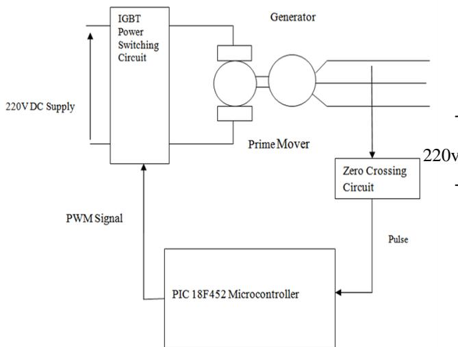
Fig 1: Frequency controlling block diagram
