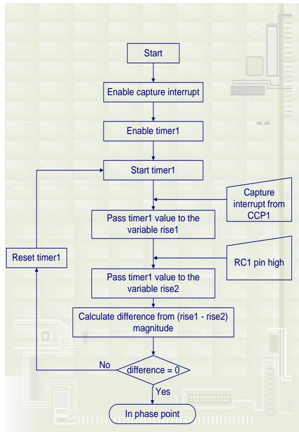
Fig 5: In phase point detection algorithm
