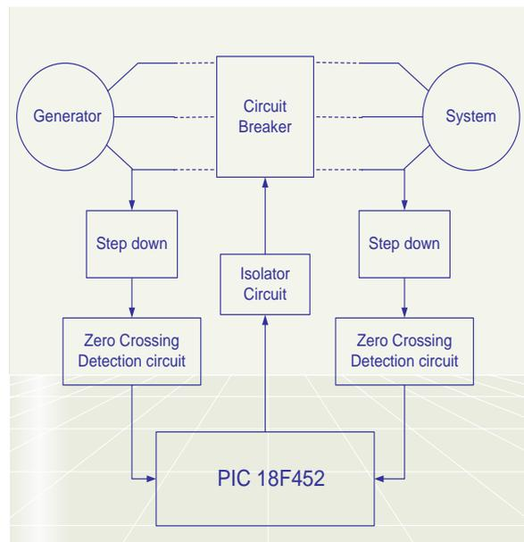
Fig 4: In phase point detecting block diagram
