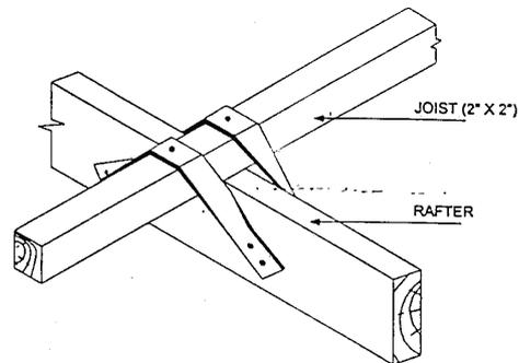
**Figure 2:** Joists should be fixed to the rafters
