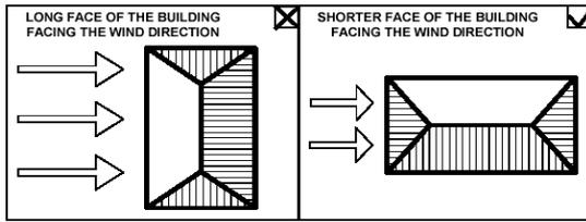
**Figure 5:** Desirable orientations for buildings
