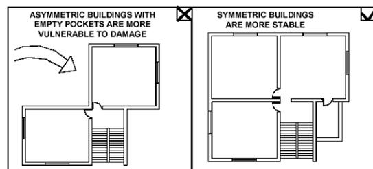
**Figure 4:** Effect of building layout
