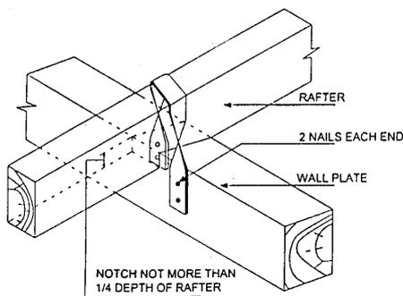
**Figure 3:** Rafters should be fixed to the wall plate
