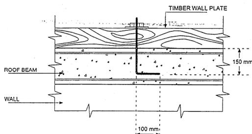
**Figure 4:** Anchoring of roof skeleton to the continuous roof beam
