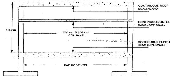
**Figure 3:** The preferred locations for tie beams
