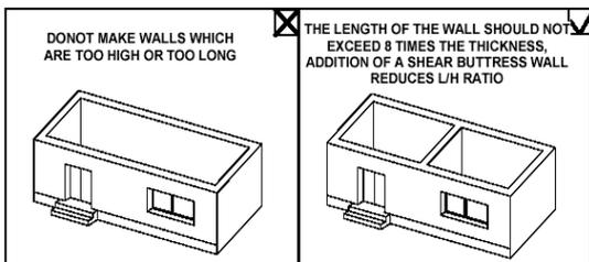
**Figure 2:** A desirable arrangement for partition walls
