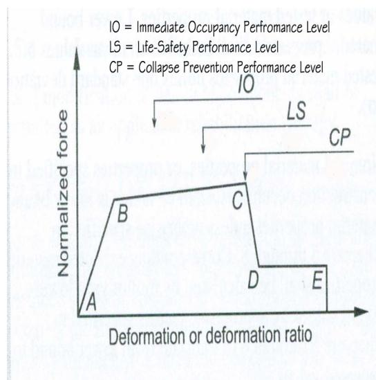
Figure 1: Acceptance Criteria of Performance levels in relation with Component Force-Deformation Curve (FEMA 356)
