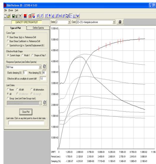
Figure 2: Demand Capacity Plot for a Perforated Shear Wall in a Push Over Analysis for a 500 year earthquake.
