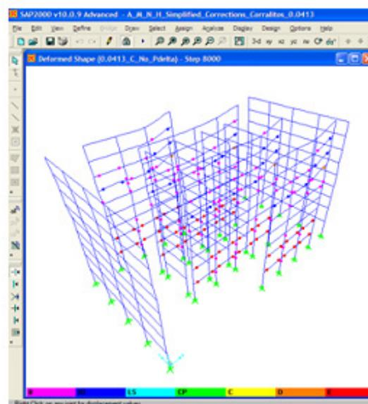
Figure 3: Results of a non linear dynamic analysis of a steel building with joint hinges formed
