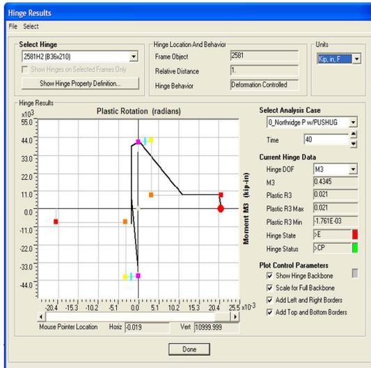
Figure 4: Plastic Moment vs. Rotation at a Moment Connections
