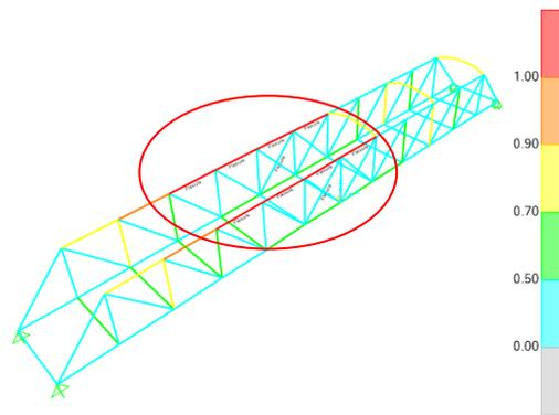
Figure 14: Demand/capacity ratios in the FE model without first three lateral bracings from the entering end
