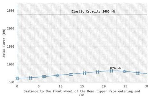
Figure 18: Axial force variation of member 7 in the FE model with all the top lateral bracings
