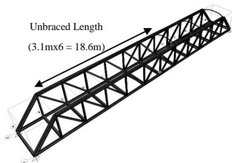
Figure 9: Unbraced length of the bridge
