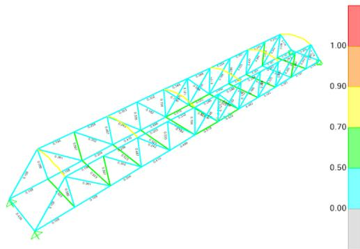
Figure 13: Demand/capacity ratios in the model with lateral bracings
