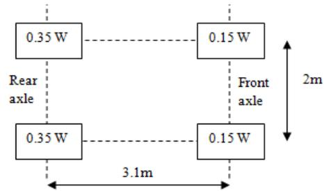
**Figure 11: Load distribution through the axles**
