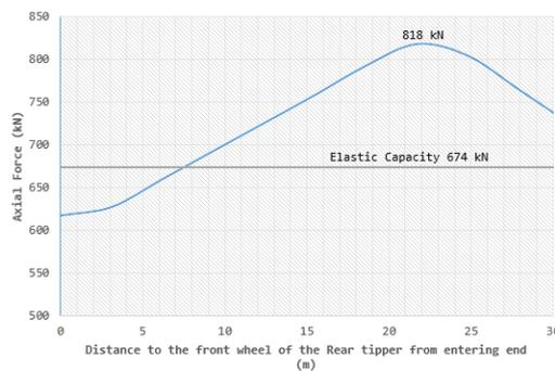
Figure 17: Axial force variation of member 7 in the FE model without top lateral bracings
