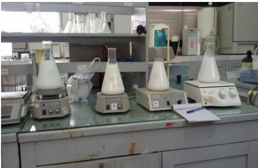
Figure 3: Synthetic Turbid Water Solution
