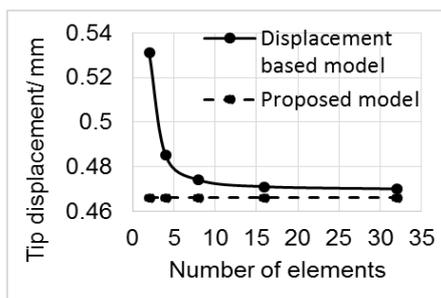
**Figure 3. Tip displacement variation with respect to number of elements**
