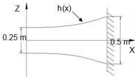
**Figure 2. Dimensions of the curved tapered beam**
