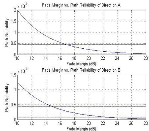
**Figure 6: Fade margin vs. path reliability**
