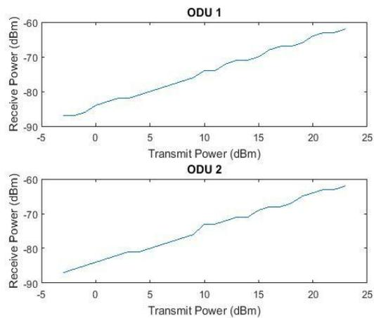
Figure 2: Transmit and receive power in practical
