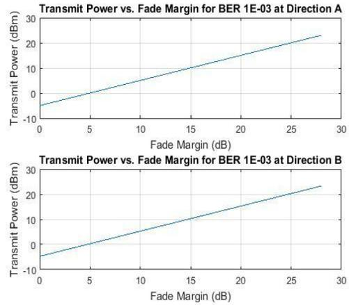
**Figure 5: Transmit power vs. fade margin for BER 1E-3**
