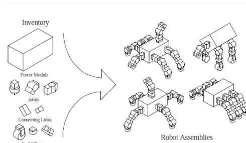
**Figure 1: A Modular Design Approach to Robotics [3]**
