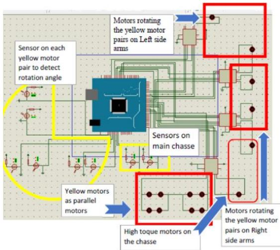
Figure 06: System block diagram of the robot. The System controls 14 motors via pulse with modulation using 4 motor drivers.
