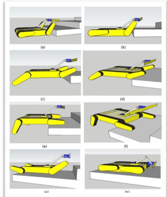
**Figure 7: Deploying side arms to overcome an obstacle in the ground**
