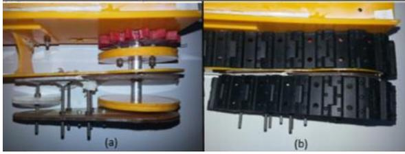
**Figure 5: Connection of main track and side arm track without (a) and with (b) the continuous track.**
