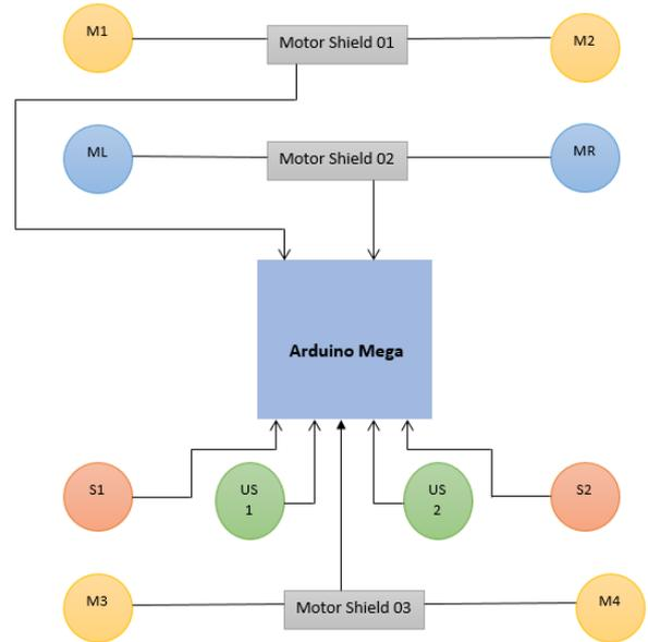
**Figure 4: System Block Diagram**
