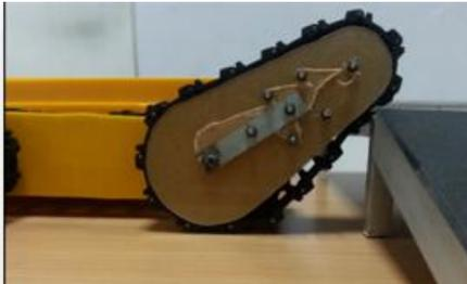
**Figure 6: Deploying side arms to overcome an obstacle in the ground**
