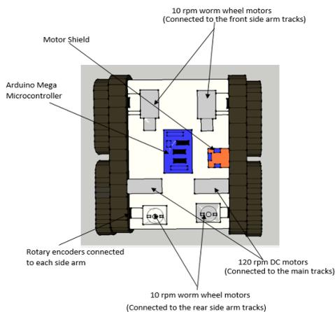
**Figure 3: Top view of the proposed UGV design**
