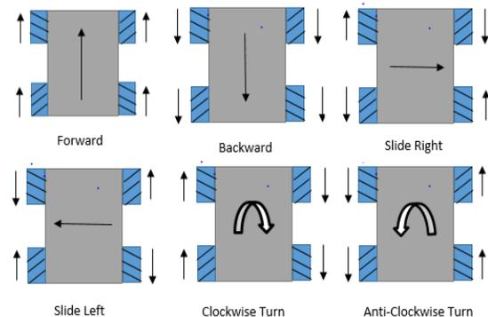
**Figure 7- Achievable Movements, by changing directions of individual wheels [3]**
