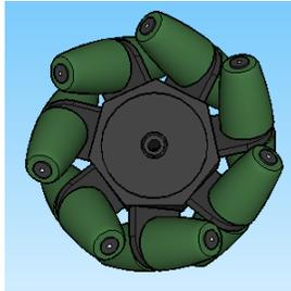
**Figure 2: basic structure of the Mecanum Wheel, consisting of seven rollers fixed at 45° to the axis of rotation**
