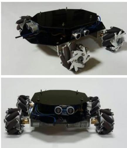
Figure 10 – Prototype Front and Top views
