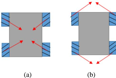
**Figure 4 (a): 1<sup>st</sup> Orientation of wheels, with rollers pointed inward, Figure 4 (b): 2<sup>nd</sup> Orientation of wheels, with rollers pointed outward.**
