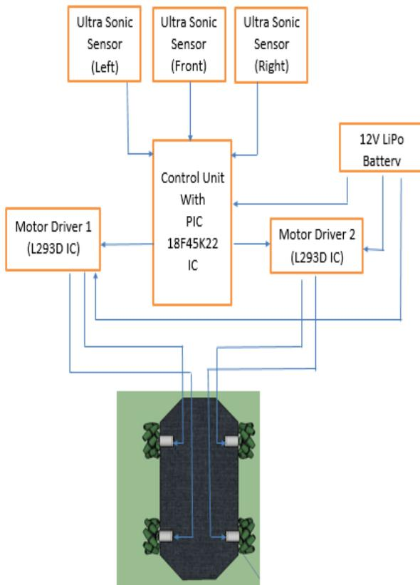
Figure 9–System Diagram
