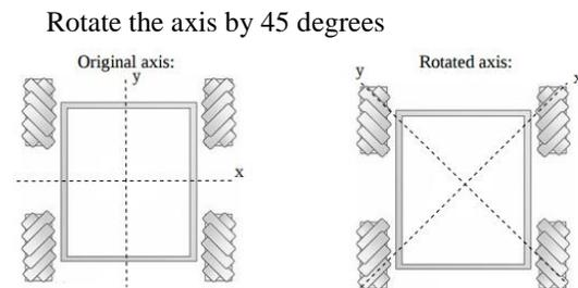
**Figure 5: Axis Orientation, highlighting the axis when rotated by 45 °**
