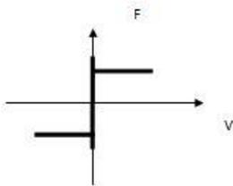
Figure 4: Coulomb friction model with stiction
