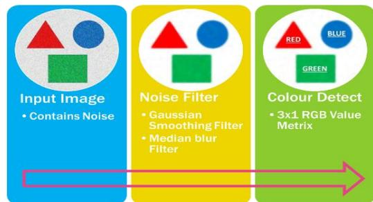
Figure 4: Image pre-processing and segmentation algorithm for colour recognition
