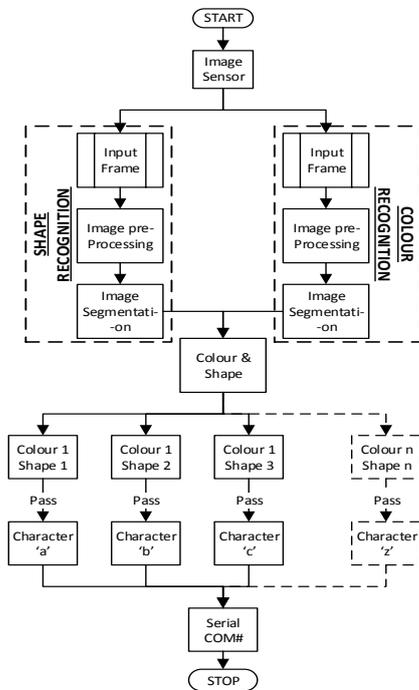
Figure 2: Image processing tool flowchart
