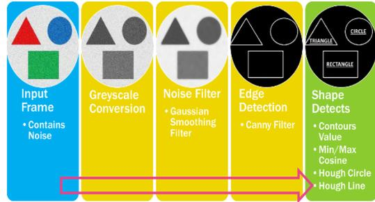
Figure 3: Image pre-processing and segmentation Algorithm for shape recognition
