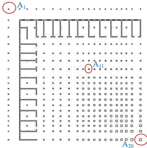
Figure 20: Quarter of the plan view at ground floor level showing column identifications
