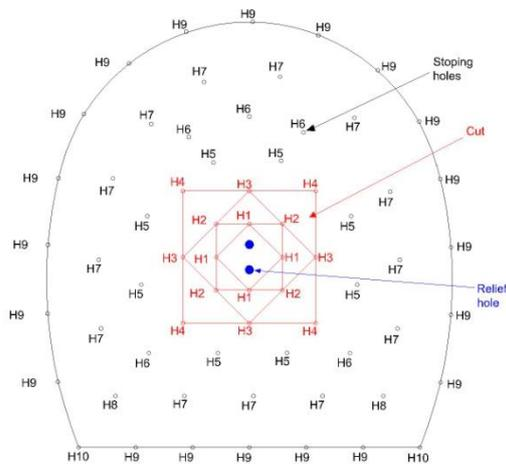
Figure 1: Drilling pattern and hole numbers
