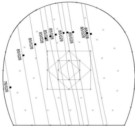
**Figure 3: Changed drilling pattern for fractured and sheared zone**
