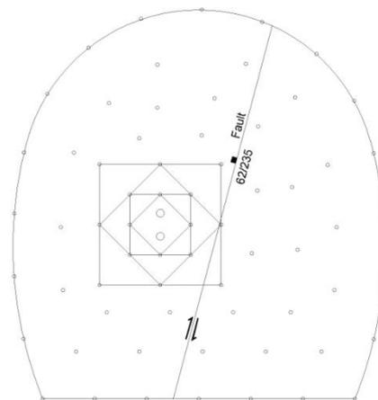
Figure 2: Changed drilling pattern for fault zone
